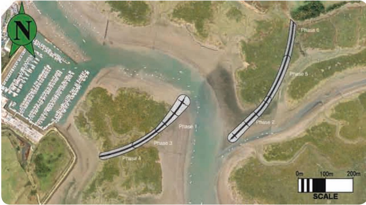
Plan of proposed breakwaters showing phasing.
